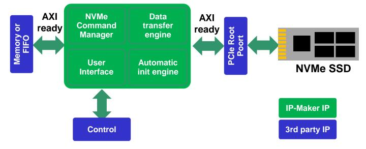
The architecture of the Host NVM Express IP is based on 4 main blocks:
