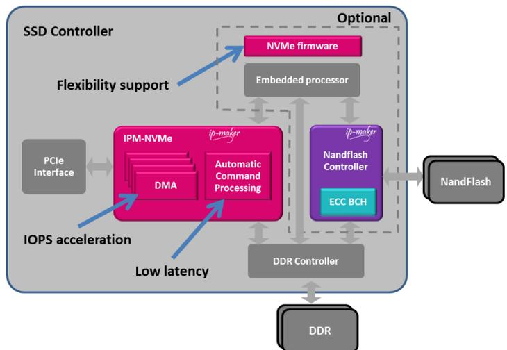
**High-performance PCIe SSD Controller Architecture**
