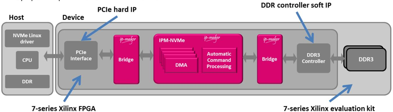
Performance: this reference design achieves **11µs** latency and **350 kIOPS** with the following configuration: PCIe Gen2 x4, QD=4, IO=4kB.
